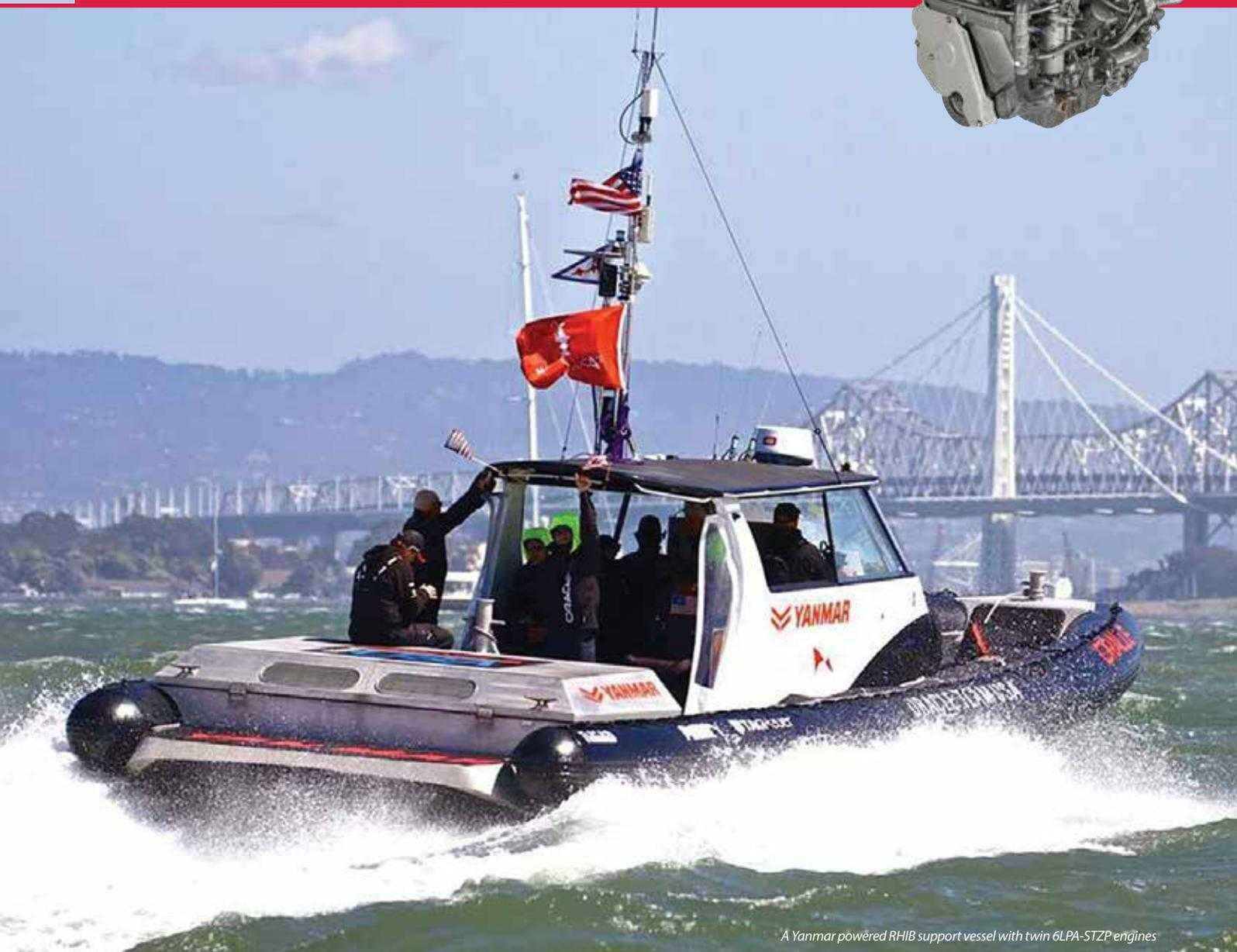
*A Yanmar powered RHIB support vessel with twin 6LPA-STZP engines*
